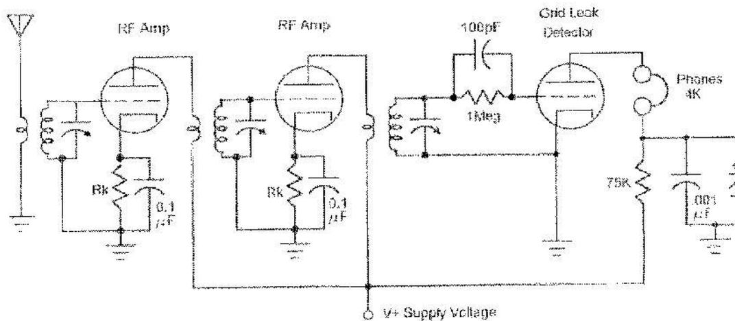
Figure 1-7: A Tuned Radio Frequency (TRF) Receiver
