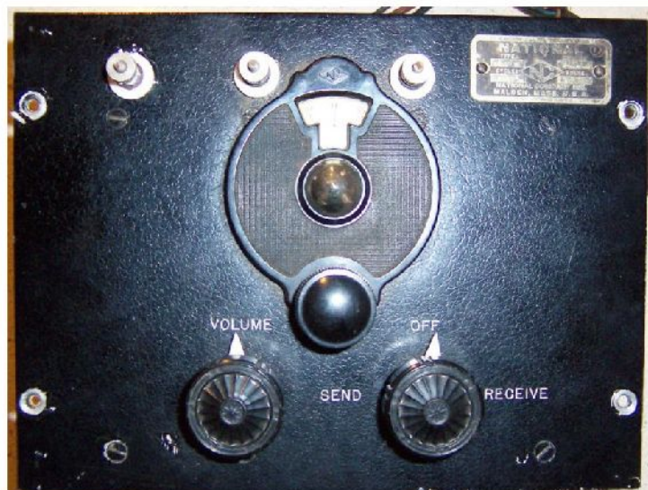
National SW-5 Five Meter Portable Transceiver – first offered in 1934 for the Five Meter band that hams had before WW2.
