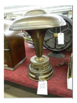
This was the 500 Executive Model. Had a typical 5 tube receiver in the base that took an external 'long wire' antenna as the radio was shielded by the base.
