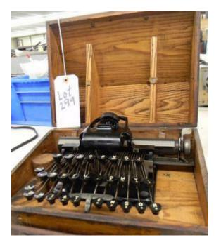
George Blickensderfer's invention dramatically reduced the complexity of the typewriter design. A typical Blick contained only 250 parts, compared to the 2,500 parts of a standard typewriter. It was much smaller, lighter and cheaper than others.
