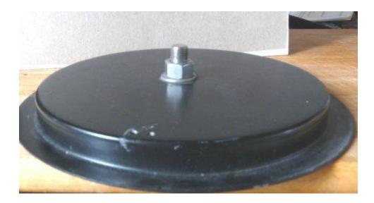
Then I obtained a dipole center piece, the sort you can use to make a dipole out of 2 hamsticks. Screwed the - side to the cap-head screw mounted in the base then Hamstick or the quick release in my case screws into the + side of the center piece and the coax with PL259 attached enters from the side .
