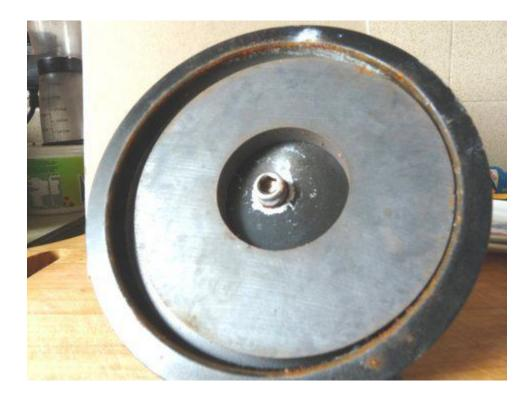
So took it all apart and inserted a stainless steel cap-head screw through the center hole (image 1 )and secured with a stainless steel nut.
