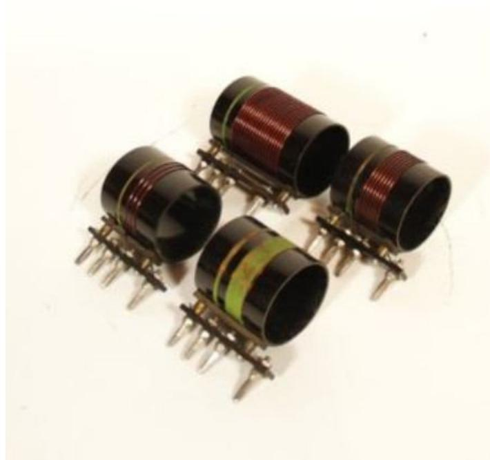
Plug in Coils for Model CS-5
