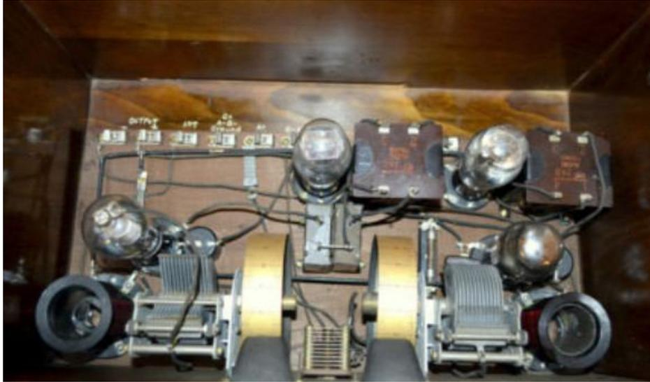
Most of these radios were sold as kits, not in a cabinet. This one appears to be a factory made unit. The set uses 4 tubes – with the RF amplifier a new 'Screen Grid' (aka Tetrode) tube which allowed higher gain. A 644SG kit sold for \$46.25 in 1928. Quite a bit of money – many hundreds of dollars in today's dollars. You could get coils to cover from 30 to 3000 meters from 10 MHz down to the below 100 KHz area.
