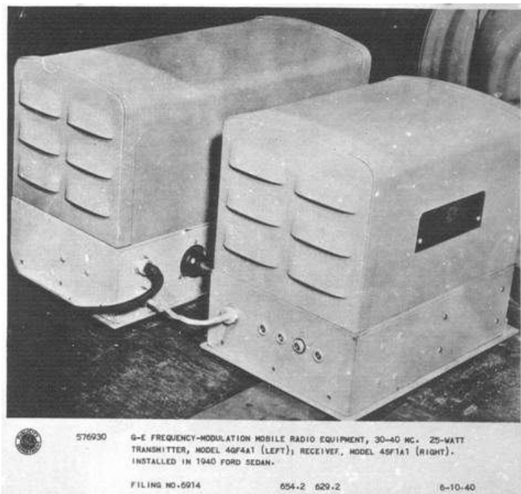
Early GE equipment. Separate large TX and RX cabinets – full of tubes
