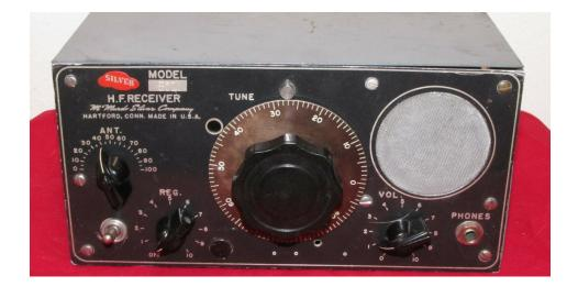
There were two versions of this. One used 1.5v tubes – for battery operation. The other used 6v tubes for operation of a separate power supply off the a/c line.
